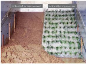
Landslide testing using precipitation testing equipment
