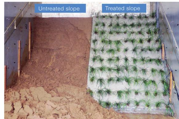
Landslide experiment using precipitation testing equipment
