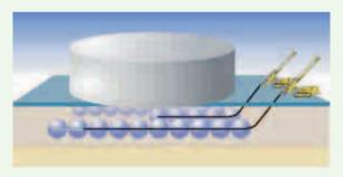
efficiencies can be achieved in soil remediation works. The navigation drilling system is ideal for remediation in areas immediately beneath active plants and factories, condominiums, gas stations and petroleum storage tanks. This system can expand remediation capabilities by facilitating the injection of materials that decompose contaminants without being hampered by structures and obstacles.
