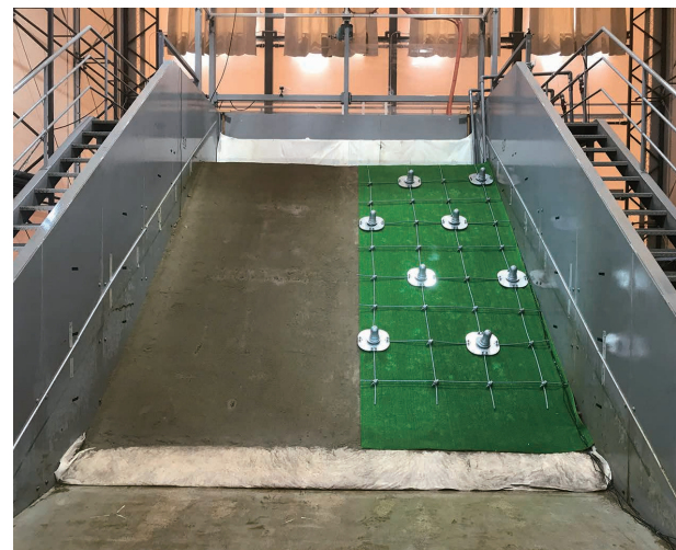
Landslide testing using precipitation testing equipment
