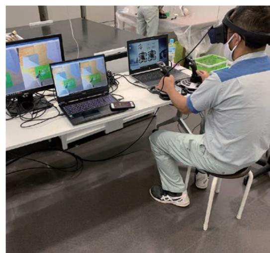
Remote operation using a head-mounted display
