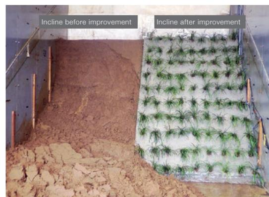
Landslide testing using precipitation testing equipment
