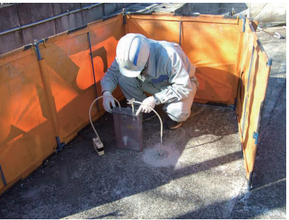
Based on the results of surveying surface pollution, including ground soil and soil gas, we survey the state of pollution at deeper levels
