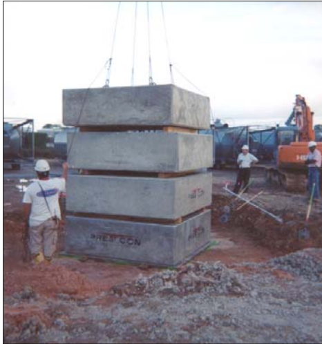
Incremental load test in progress
