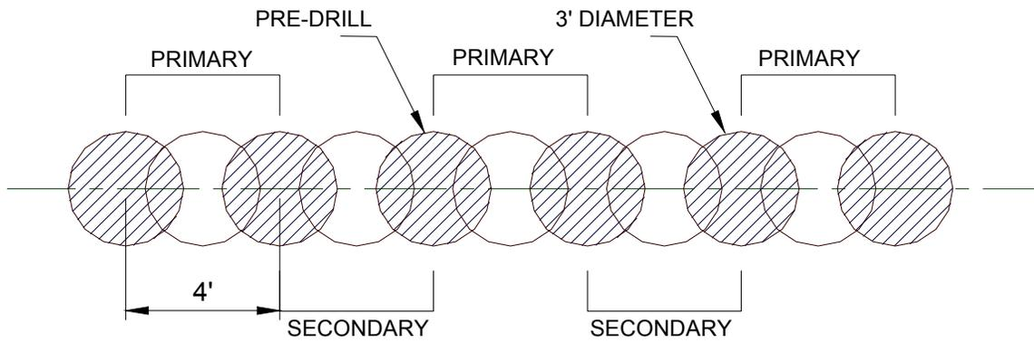
Figure 3a: Soil-Cement Cutoff Wall
