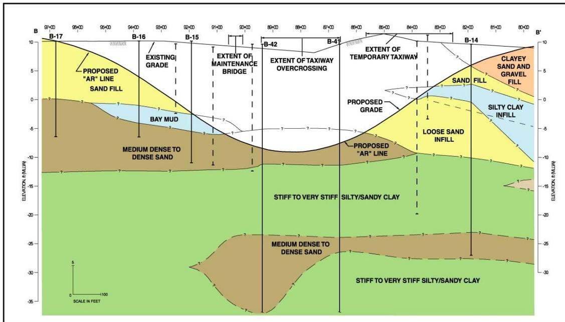
Figure 9: Idealized Soil Profile (Courtesy of Geomatrix Consultants)
