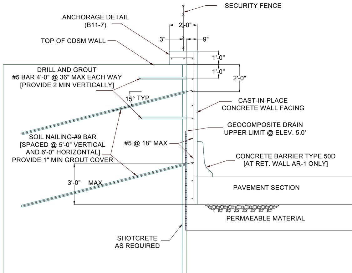
Figure 10: Design of CDSM Gravity Wall
