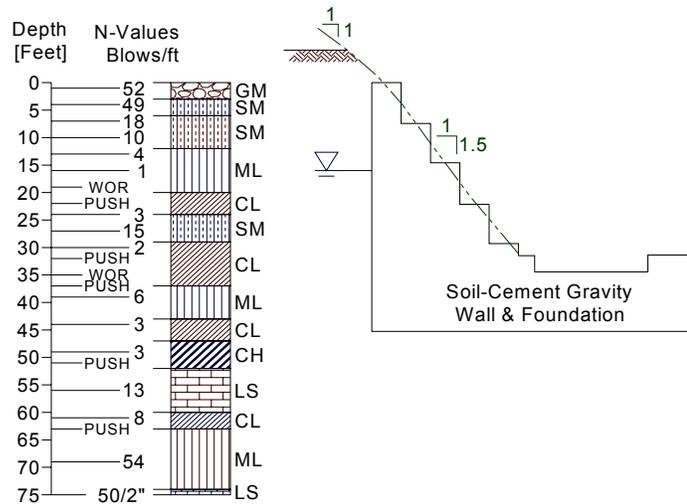
Figure 13: Representative Boring Log and Subsurface
