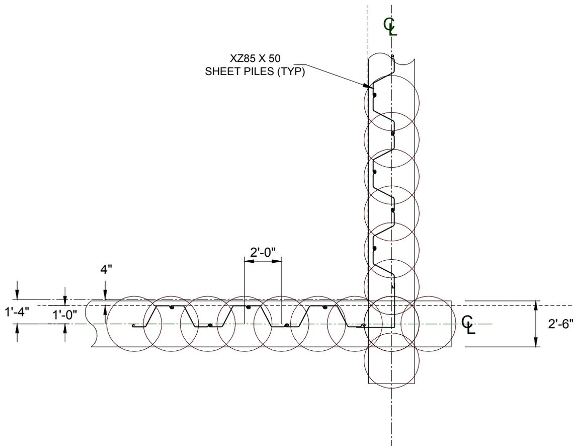
Figure 3b: Soil-Cement Excavation Support Wall
