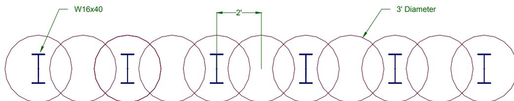
Figure 7b: Reinforcing Layout
