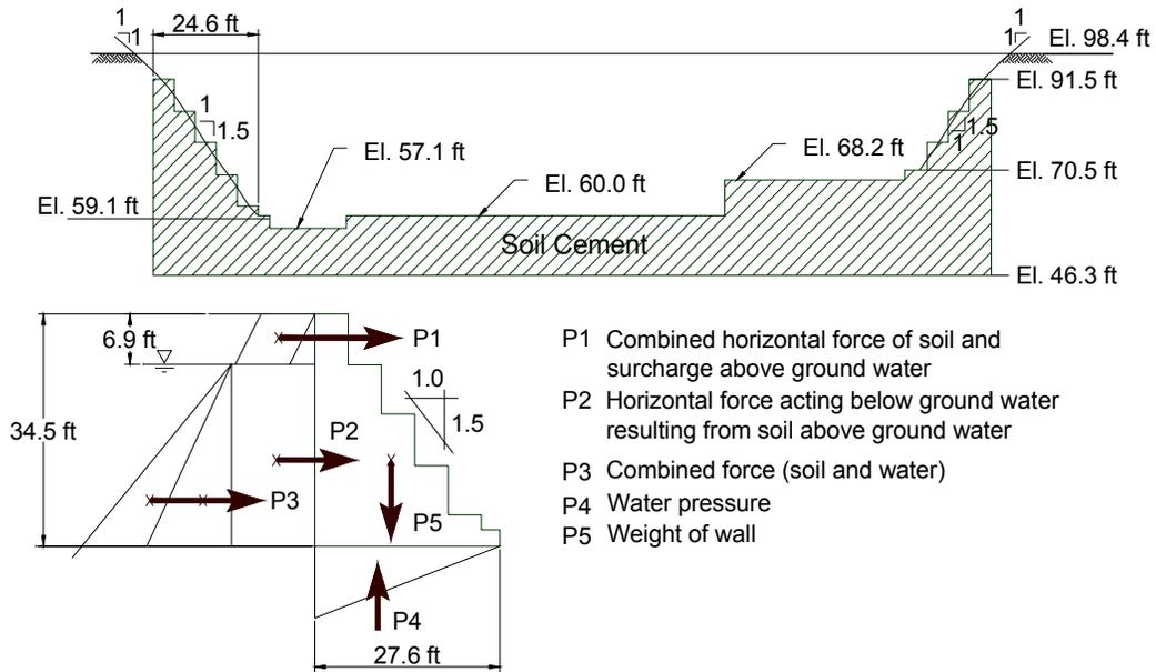
Figure 15: Cross Section A-A (Courtesy of Bechtel Corporation & EERI)
