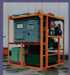
SL mixing plant
