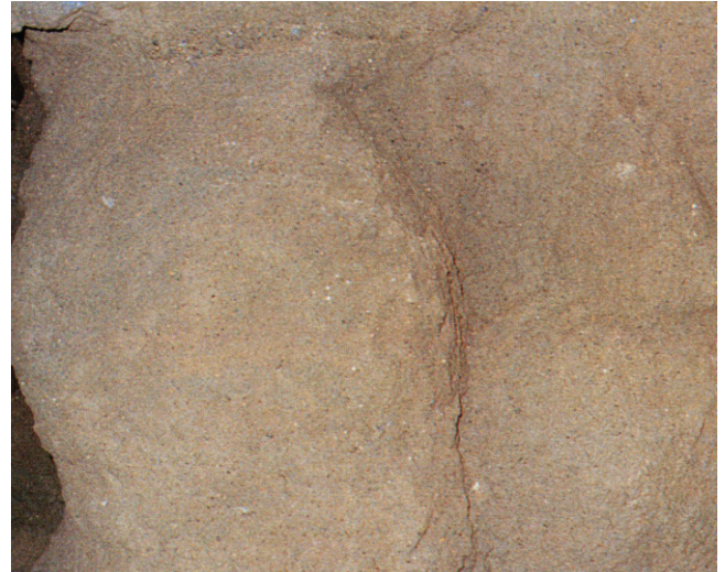
Solidified sand-grout mass by permeation grouting
