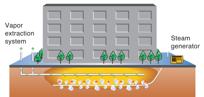
Steam is injected to vaporize VOCs, which are collected through extraction well by vapor extraction system.
