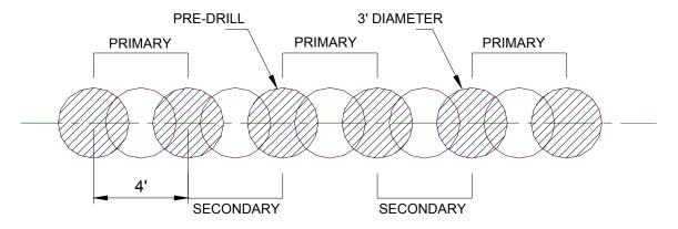
Figure 3a: Soil-Cement Cutoff Wall
