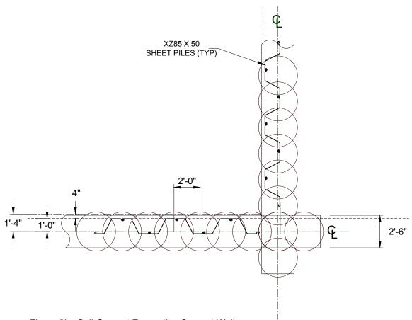
Figure 3b: Soil-Cement Excavation Support Wall
