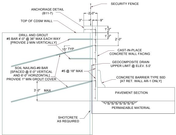
Figure 10: Design of CDSM Gravity Wall
