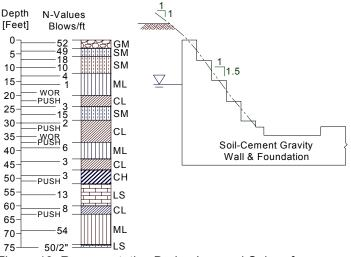
Figure 13: Representative Boring Log and Subsurface
