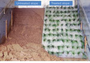
Landslide experiment using precipitation testing equipment
